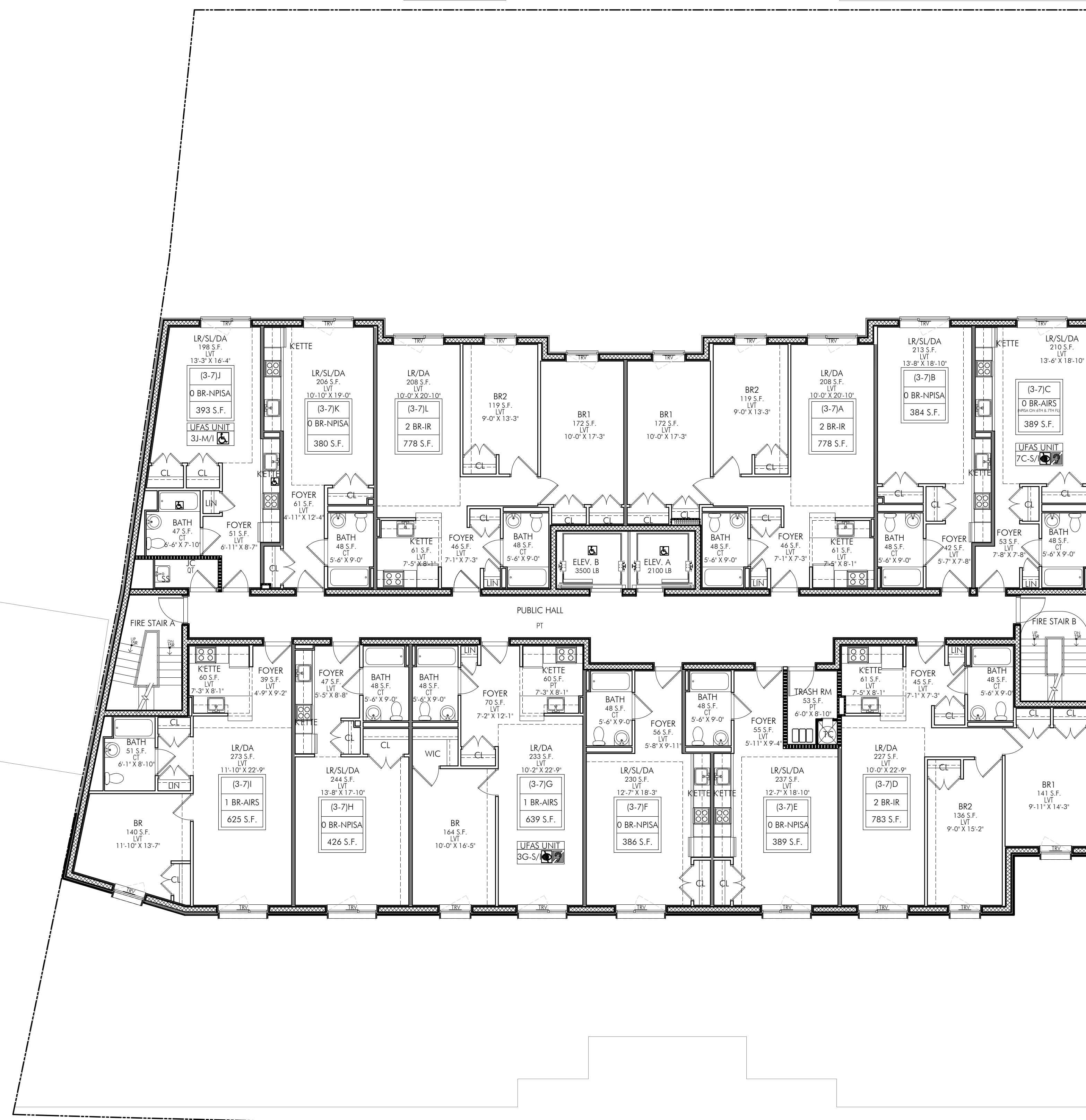
1 TYPICAL (3RD - 7TH) FLOOR PLAN 1/8"=1'-0"
