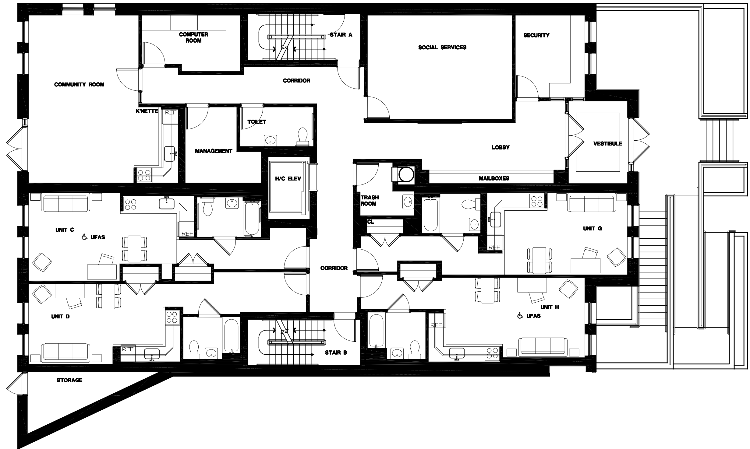
FIRST FLOOR PLAN SCALE: 1/8"=1'-0"
